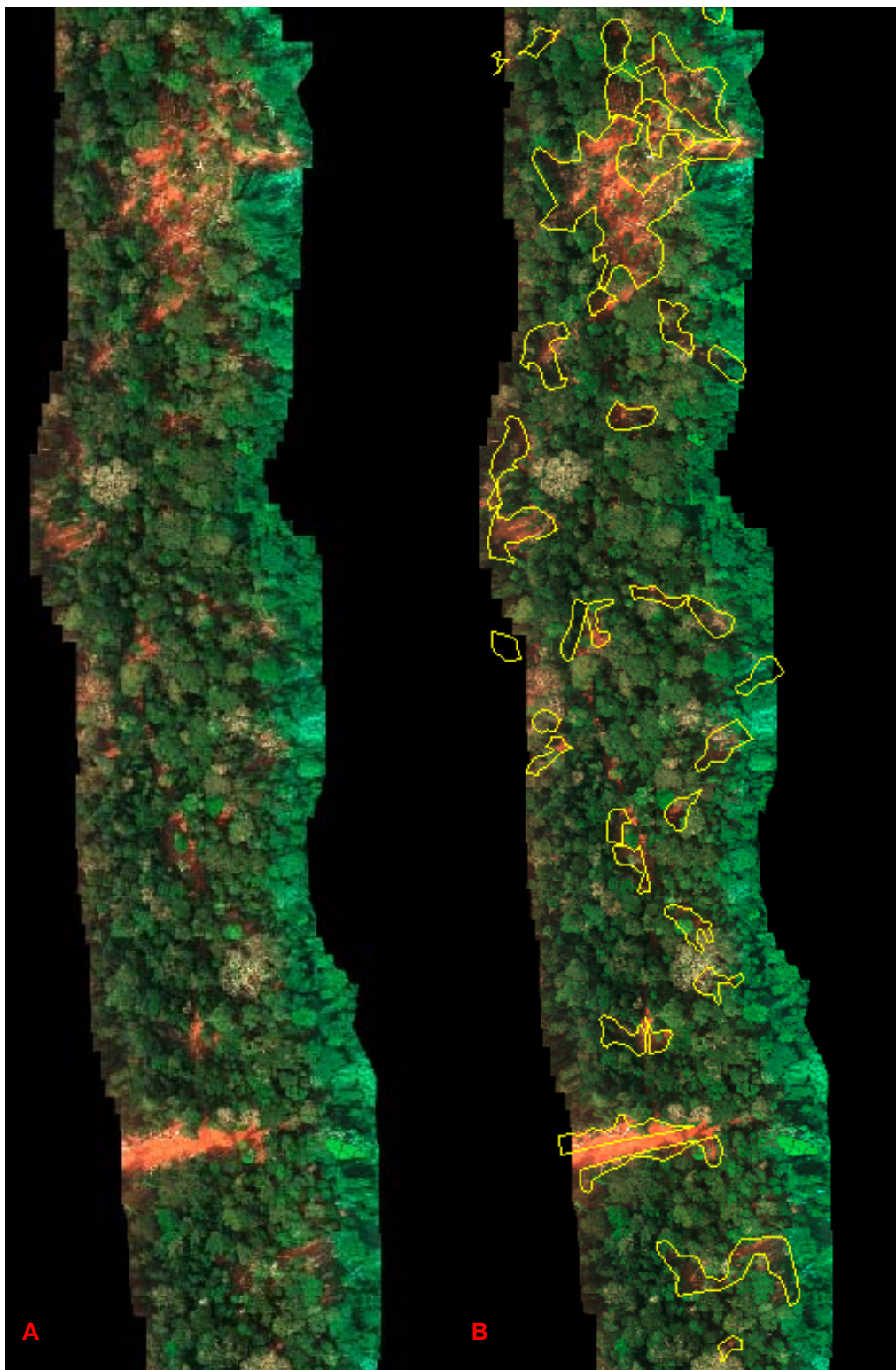
Figure 13. Strips of aerial imagery showing logging damage, in B the areas of damage are delineated. The imagery is designed to be seen in three dimensions and so some of the polygons are offset when seen in two dimensions
