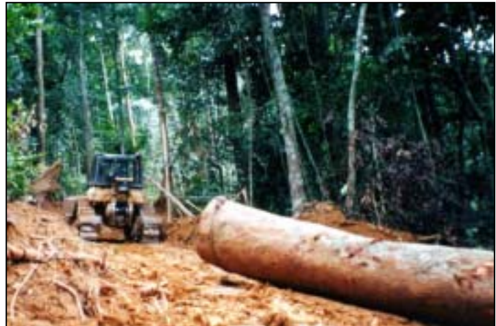
Photo 23. In addition to Timberjack 480 rubber-tired skidders, SBL also uses Caterpillar 527 high-sprocket tracked skidders as shown here.
