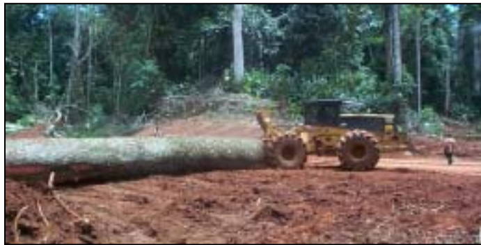
Photo 10. Caterpillar 545 skidder delivering a large log to a roadside landing on the CIB concession.
