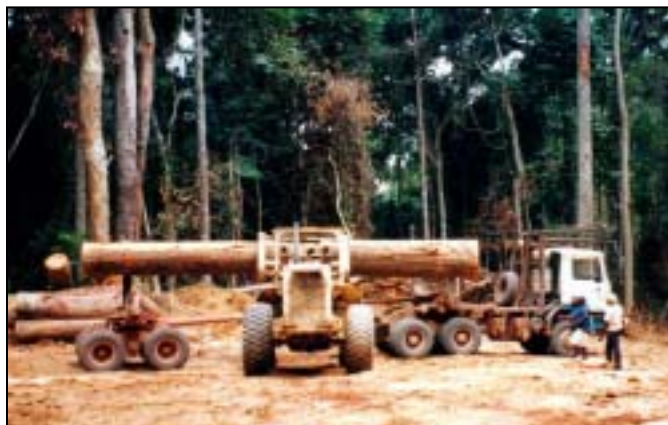
Photo 21. At a landing on the SBL concession, a front-end loader places a log on a logging truck.
