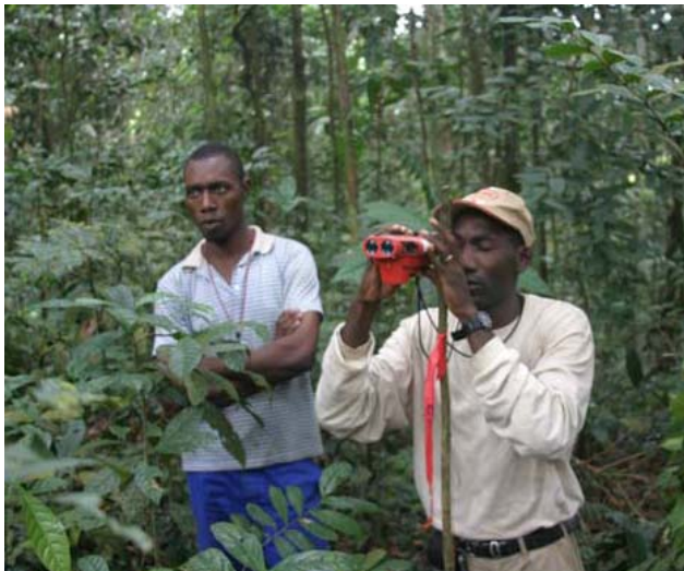
Figure 2: Line sighting and horizontal distance measurement using a laser range finder
