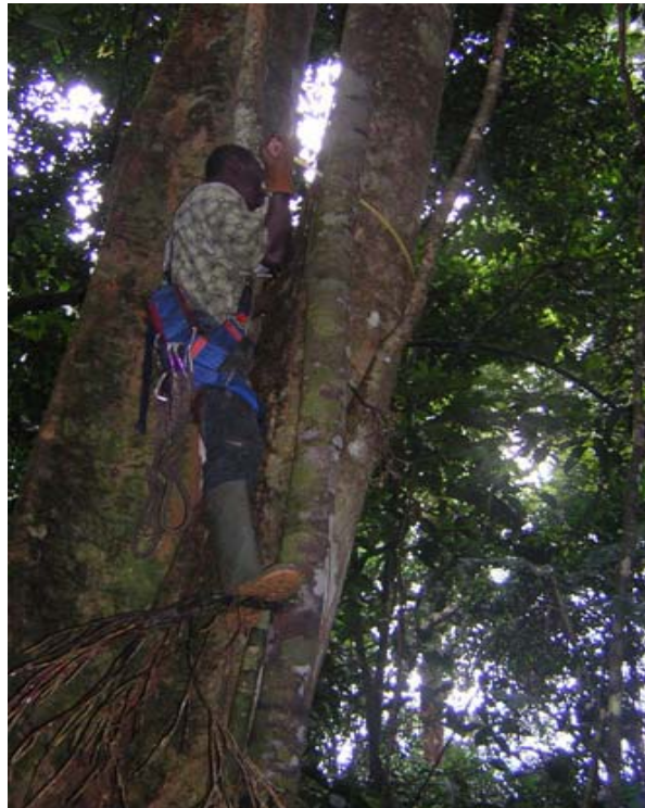
Figure 4. Measuring tree diameter at reference height (drh)
