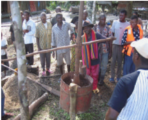
Figure 2. Bomongo association representatives demonstrate a press for extracting oil from palm nuts. R. Alexander photo
