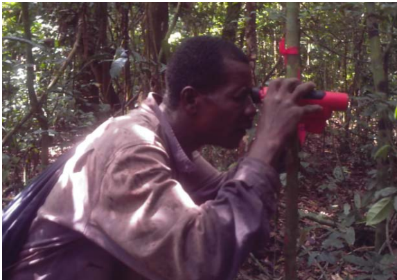
Figure 4: Line sighting and horizontal distance measurement using a laser range finder.
